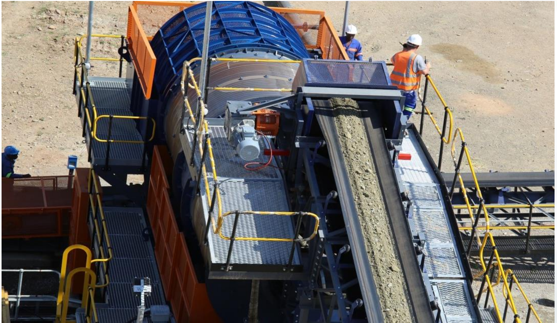
Kimberlite Ore from the Primary Crusher being fed into the new Primary Scrubber
