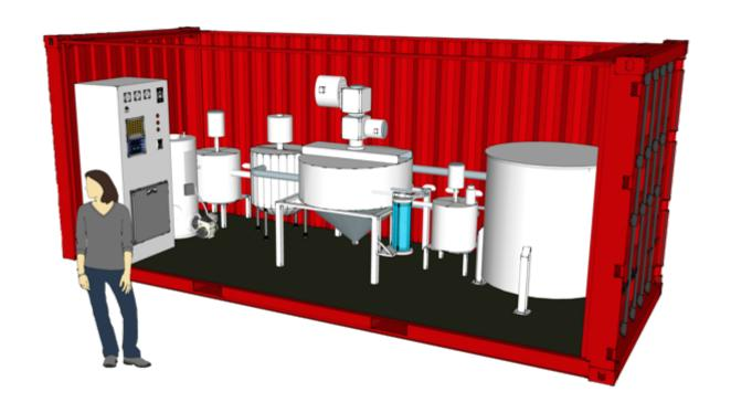
Our plant was designed to fit into a 40' shipping container so that it can be deployed to the optimum location for supply & integration into a manufacturing production process.
