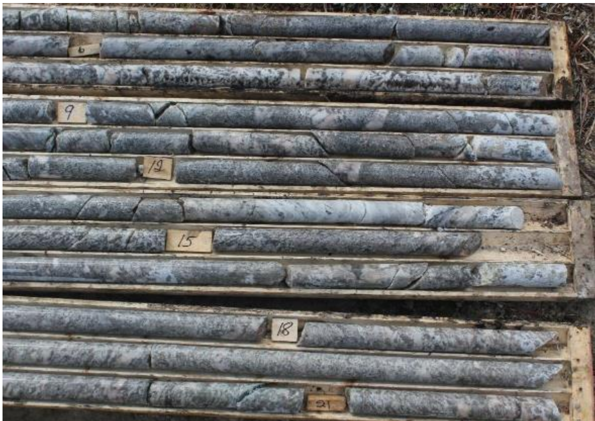
Figure 3. Drill core from the McCombe Pegmatite at the Root Lake Project showing multiple intersections of spodumene mineralisation.
