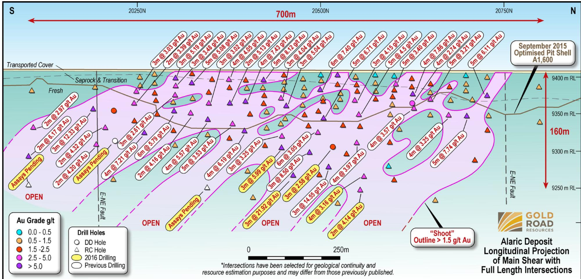
Figure 2: Alaric Longitudinal Projection looking west, illustrating locations of full length intersections on the Main Shear and high-grade extensions below the existing open pit resource with selected high-grade intersections labelled and an interpreted "Shoot" outline > 1.5 g/t. Mineralisation has only been drilled to a depth approximately 160 metres below surface, footwall lithology is basalt.
