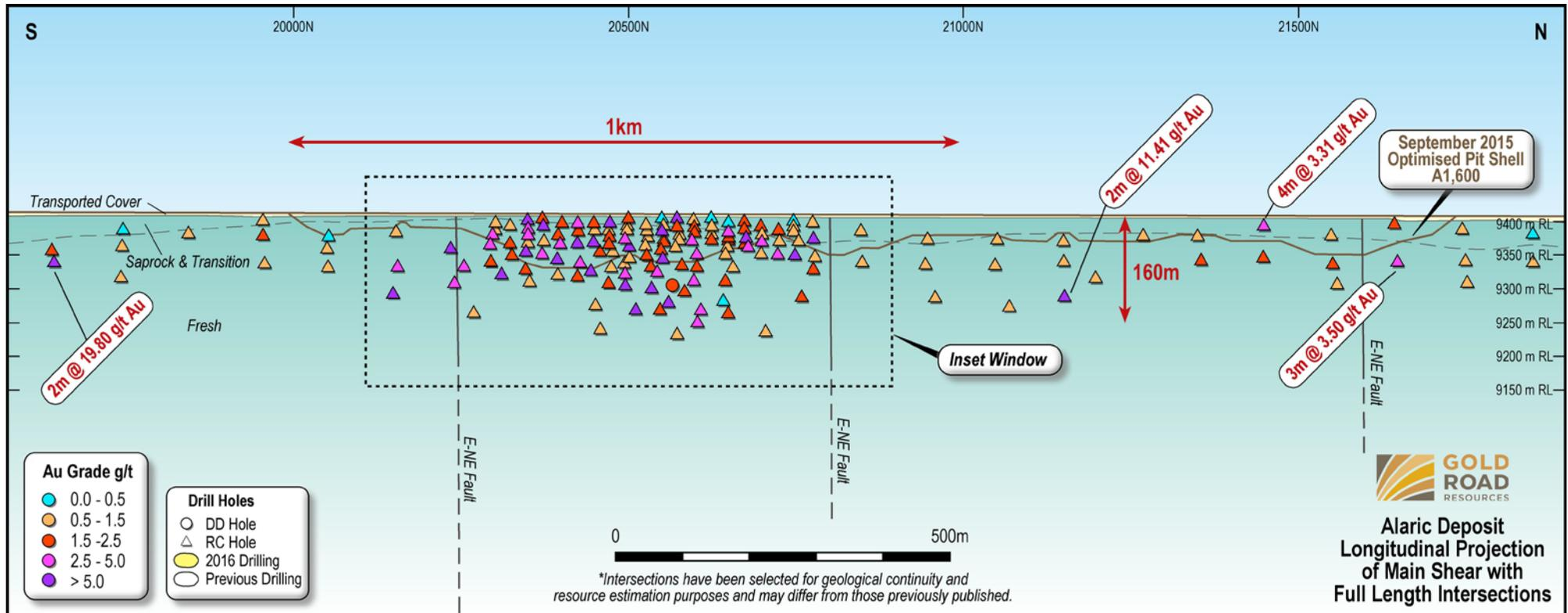
**Figure 3:** Alaric Longitudinal Projection looking west, the Inset Window shows the location of Figure 2. The figure illustrates the locations of full length intersections on the Main Shear over the full strike length of the open pit resource with selected high-grade intersections north and south of the Inset Window labelled to demonstrate the greater strike potential.
