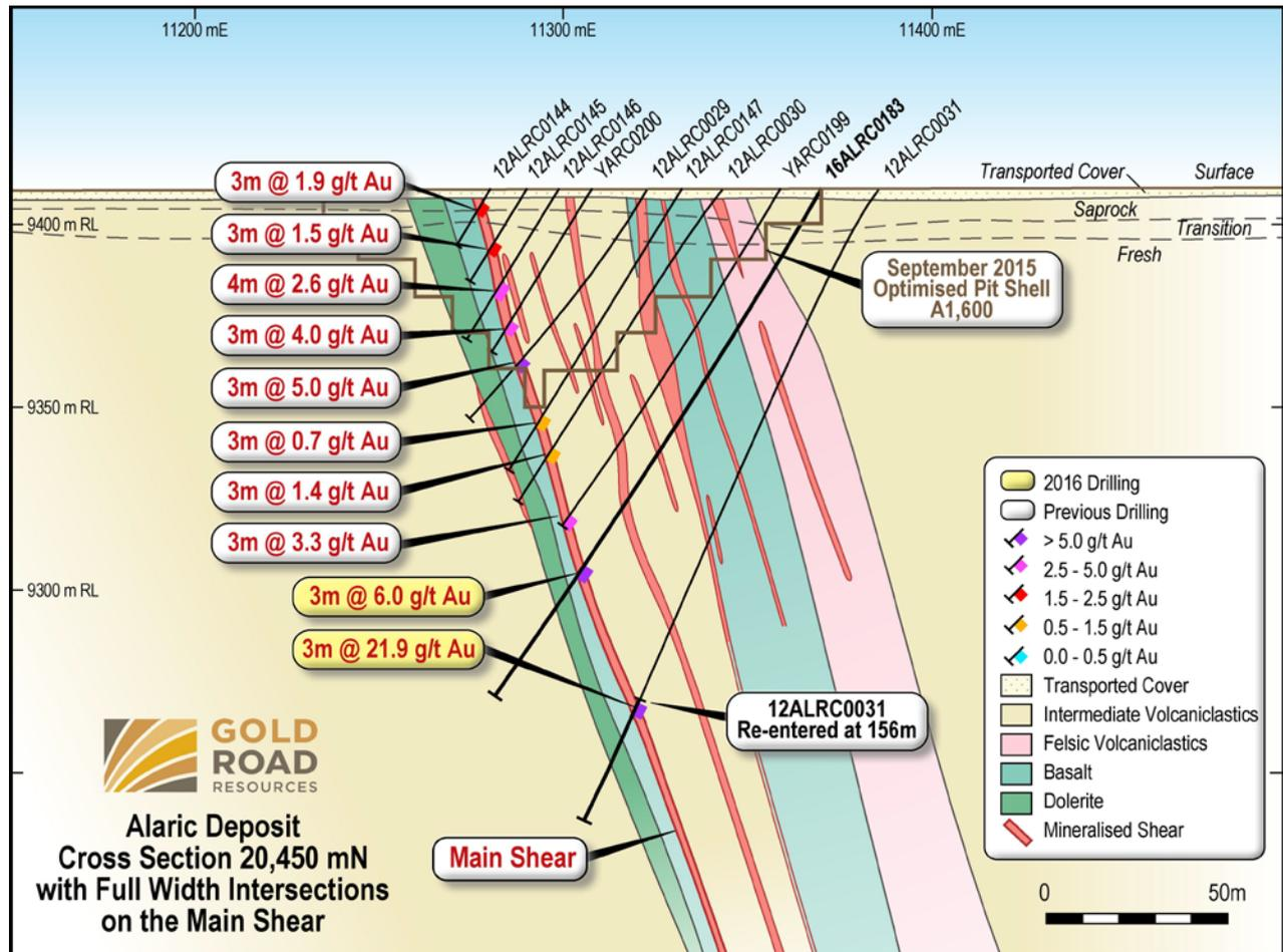
Figure 1: Alaric cross section 20,450 mN showing the geological interpretation with all full length intersections on the Main Shear labelled.
