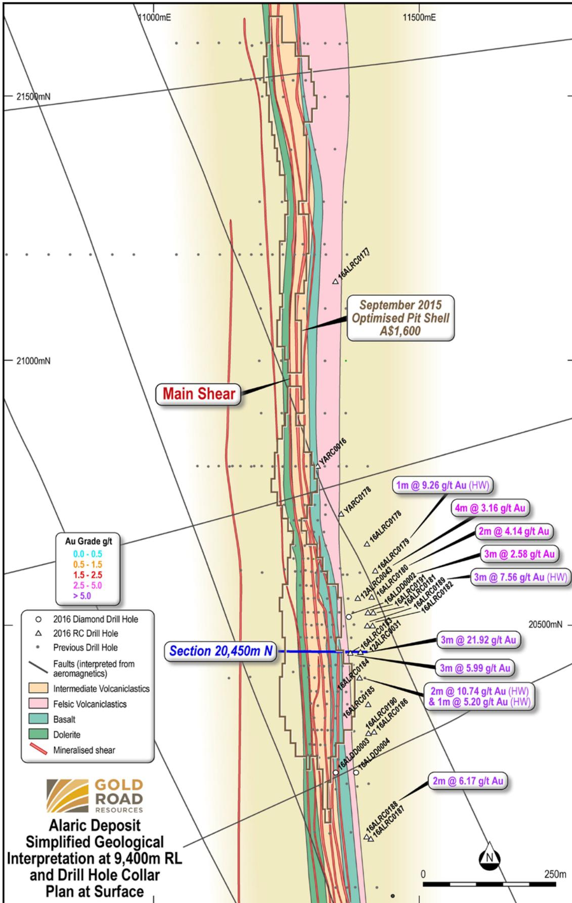
Figure 4: Alaric simplified Geological Interpretation, 2016 drill hole collars and full length intersections on the Main Shear > 2.5 g/t Au and significant Hangingwall Structures (HW) highlighted.
