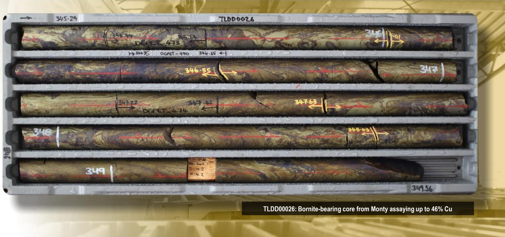
TLDD00026: Bornite-bearing core from Monty assaying up to 46% Cu
