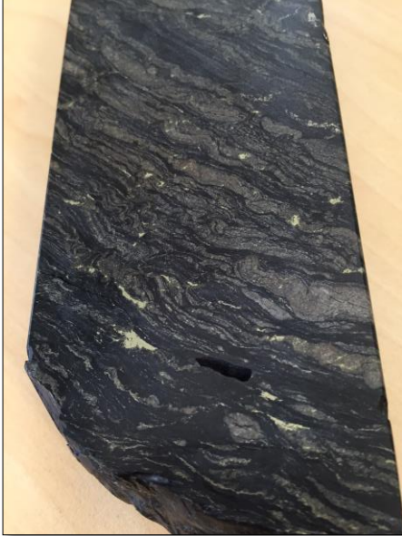
Photo 1: Disseminated chalcopyrite in carbonaceous shale EPT 2282 ~259.5m downhole (1.0%Cu) Core width ~60mm
