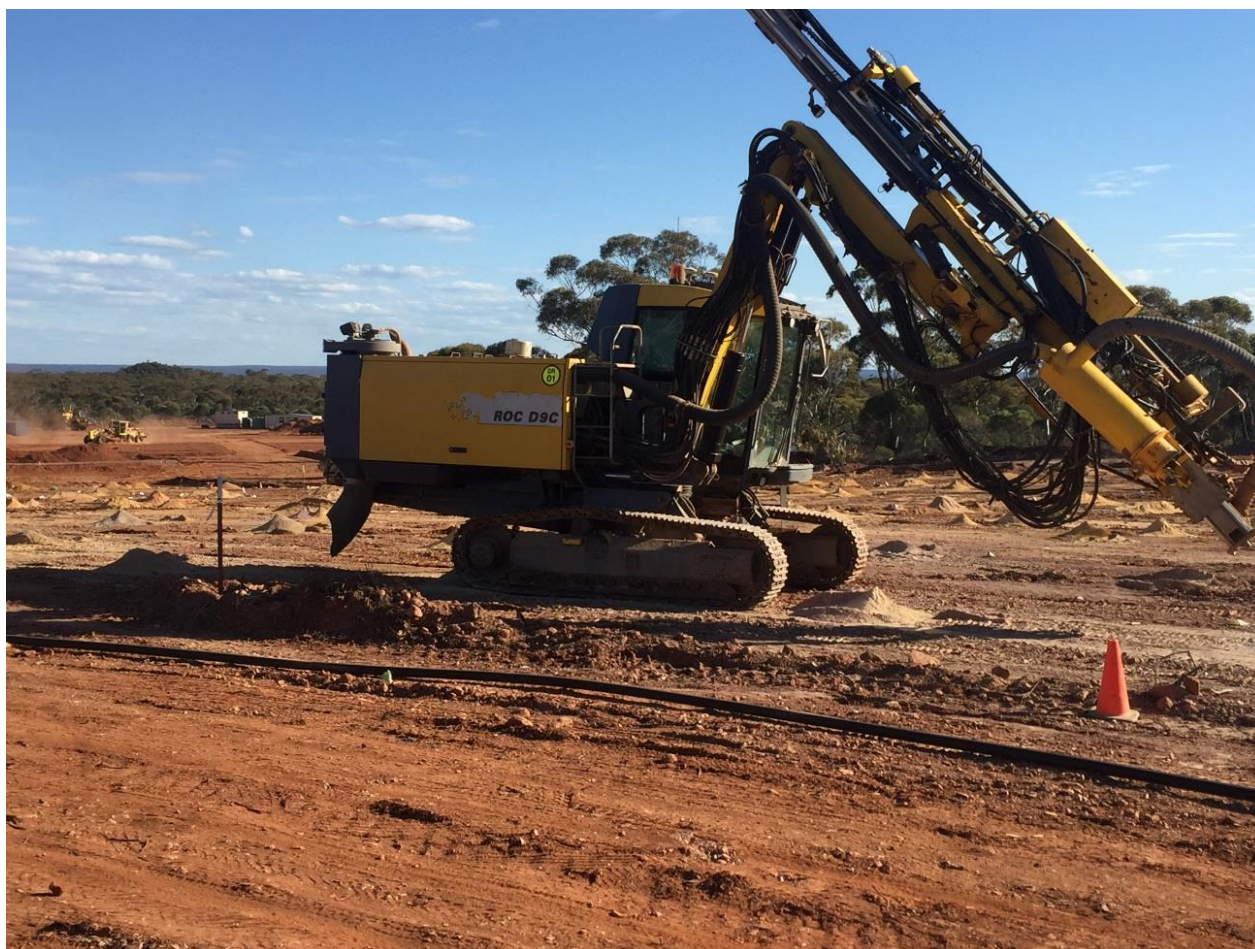
Figure 2: Trial pit blast hole drilling
