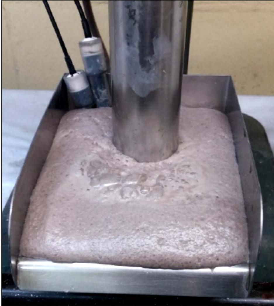
Figure 1: Pegmatite flotation test
