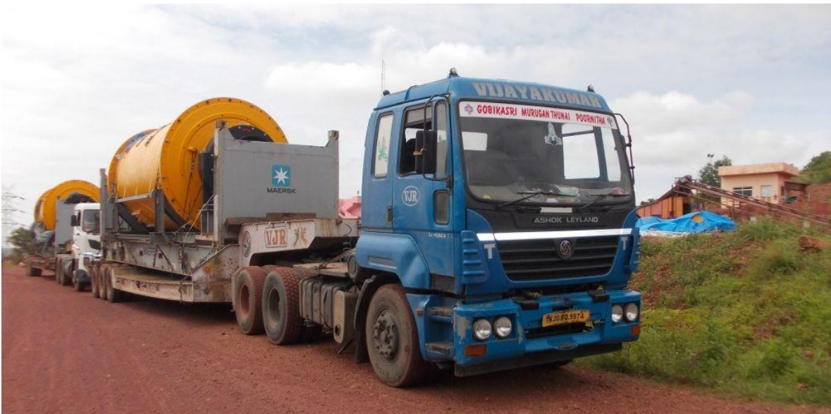
Ball Mills Arrival On Site
