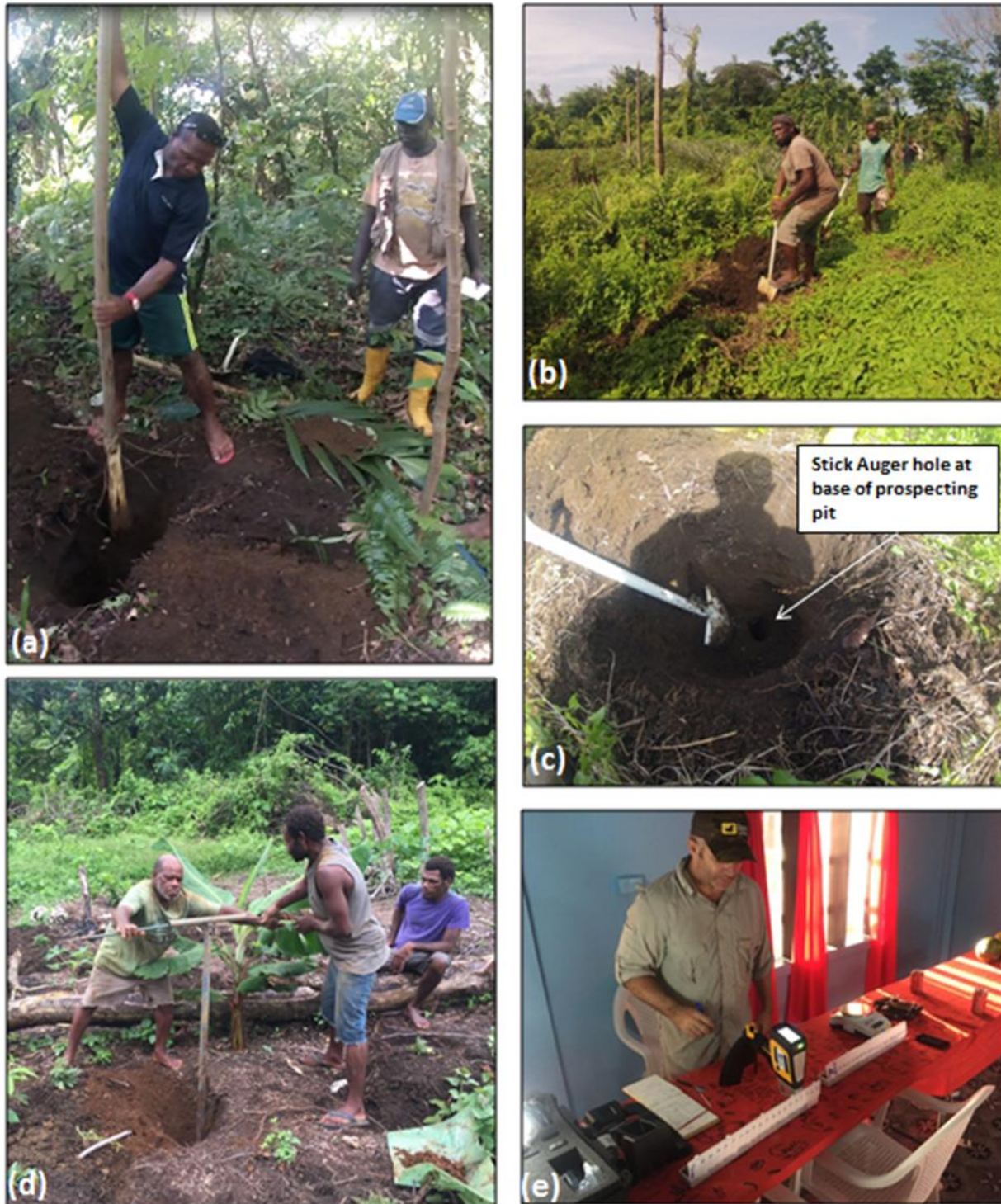
Figure 3: (a) Stick Auger being used for sampling bauxite profile. (b) Land Owner assisting prospecting on his own farm. (c) Stick Auger hole at bottom of hand dug prospecting pit. (d) Conventional Hand-Auger sampling. (e) Field analysis using hand-held XRF.
