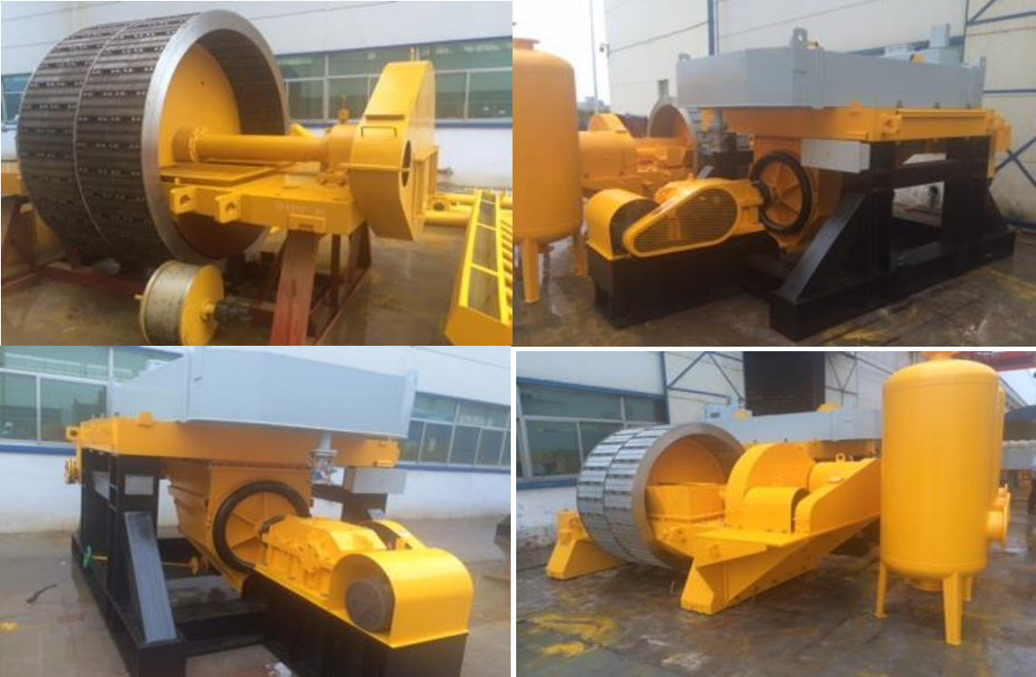
Magnetic separation equipment painted post testing and ready for packing
