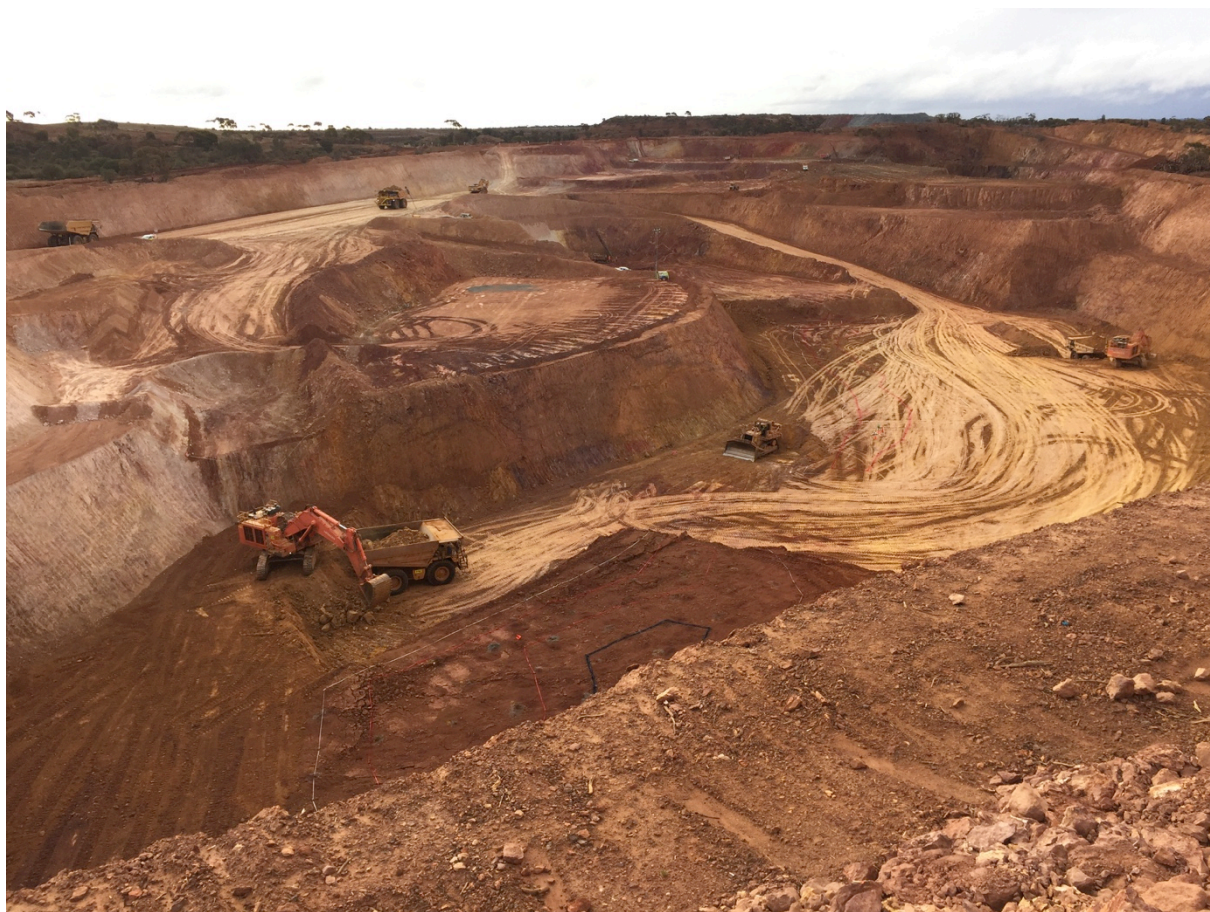
Figure 3: Zoroastrian Central Pit – looking south to north showing ore mark-up in foreground and mining activity in the Southern and Northern sub-pits (photograph date 13/06/2016)
