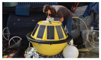
Wave monitoring buoy being prepared for deployment in Mauritius by Carnegie Analysis Engineer, Jess Kolbusz
