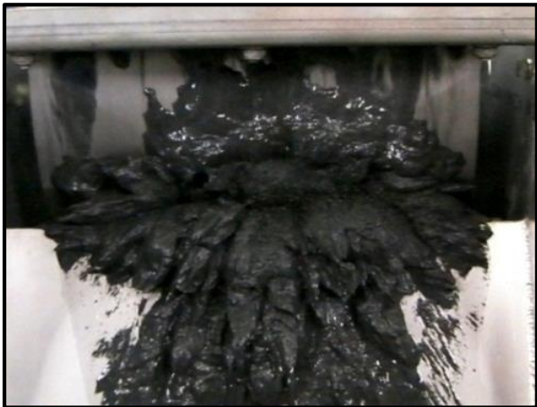
45% rejection at first magnetic separation
