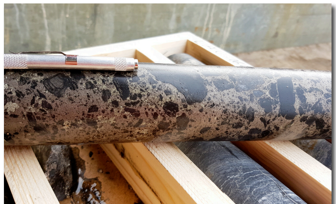
Figure 7 Matrix-supported hydrothermal breccia with graphite clasts intercepted in LAU16001 (~18.00m) at Lautakoski prospect, Jalkunen Project.
