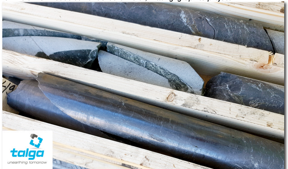
Figure 1 High grade graphite from the 'hangingwall graphite unit' intercepted in drillhole NUN16006 at Nunasvaara North, Vittangi graphite project.
