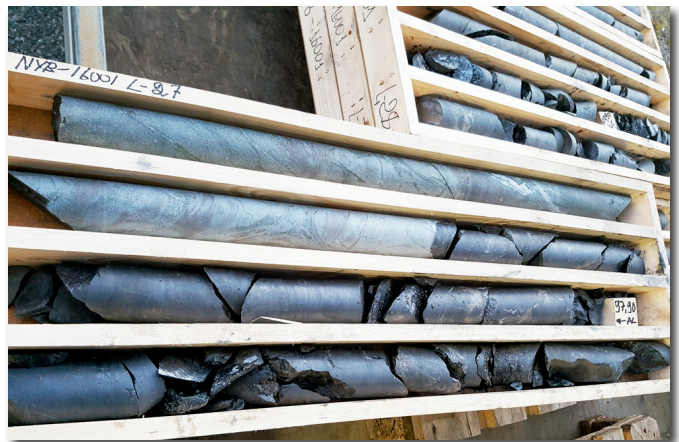
Figure 7 Matrix-supported hydrothermal breccia with graphite clasts intercepted in LAU16001 (~18.00m) at Lautakoski prospect, Jalkunen Project.
