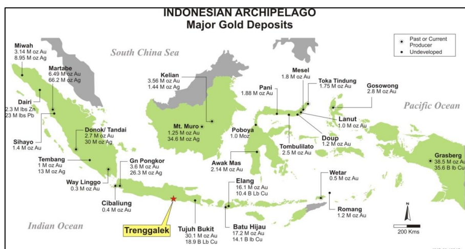
Figure 1. Trenggalek Project location & major gold and base metal deposits in Indonesia
