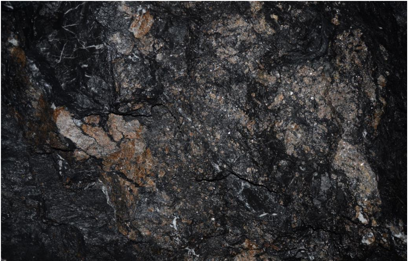
Figure 2: High-grade zinc mineralisation in cross-cut on the 940 level from where bulk samples for Ore Sorting and Locked Cycle test work have been extracted
