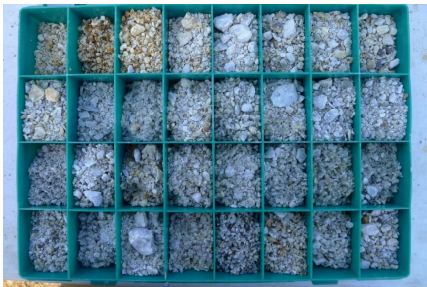
Figure 1: Chip tray showing petalite-bearing pegmatite. Each compartment represents one metre of drilling.
