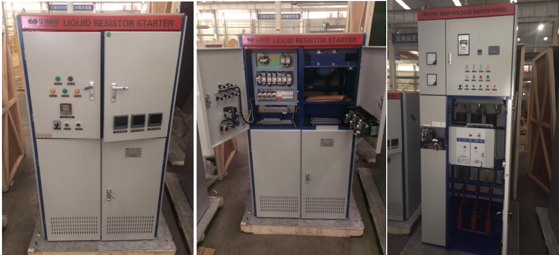
Liquid Resistor starters and high voltage switch panels being prepared for shipping
