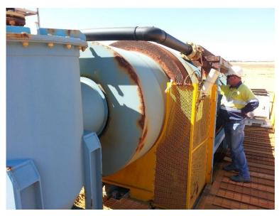
Figure 12 – PCP Trommel in Poor Condition. Significant Corrosion through the Barrel.
