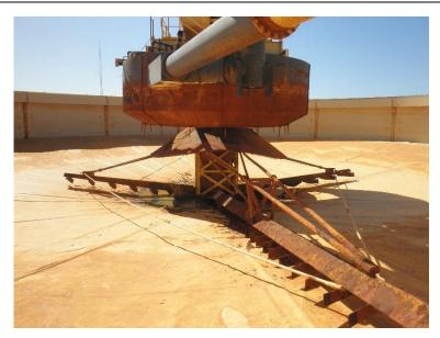
Figure 22 - PCP Thickener in Poor Condition. Significant Corrosion and Collapsed Feed Well Base
