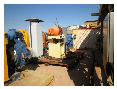
Figure 9 – Multiple Booster Pumps All in Good to Very Good Condition
