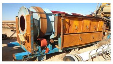
Figure 8 – SMU Trommel in Good Condition. Only the Guards Showing Surface Corrosion.
