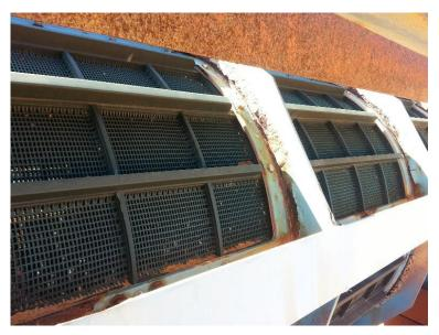
Figure 13 – PCP Trommel in Poor Condition, Significant Corrosion Through the Screen Mounts.
