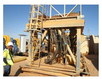
Figure 5 – SMU Trommel Support and Electrical Cables in Good Condition
