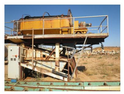
Figure 21 – CONS Trommel in Poor Condition.
