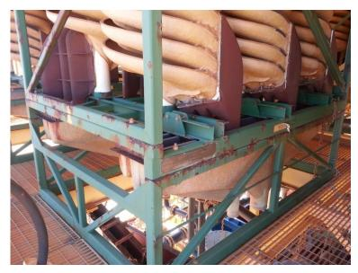
Figure 14 – PCP Spirals Are Reasonable, However the Spiral Frames Have Significant Corrosion
