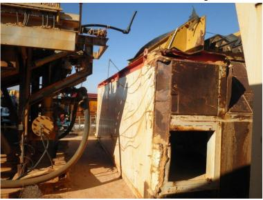
Figure 4 – SMU Grizzly Showing Damage
