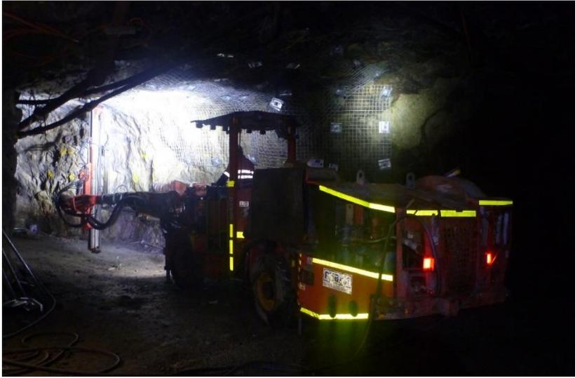
**Photo 4: Pybar jumbo at work in Golden Age Pump Station**
