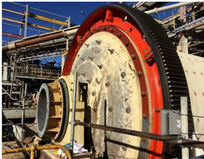
Photo 6: Mill 2 girth gear installed
