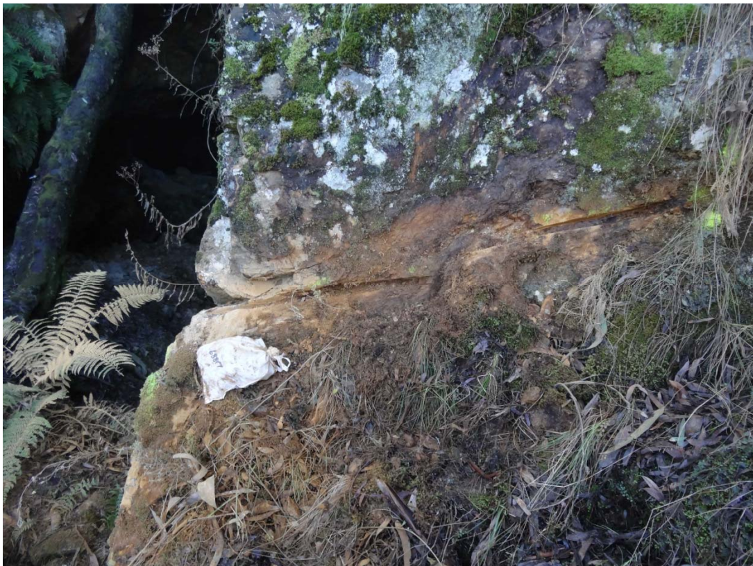
Photograph 1. Completed saw cut channel sample 68817 (Looking North West). Hanging wall sediments east of Main Fairleys shear (open slope left of photograph, mined in lower open cut).
