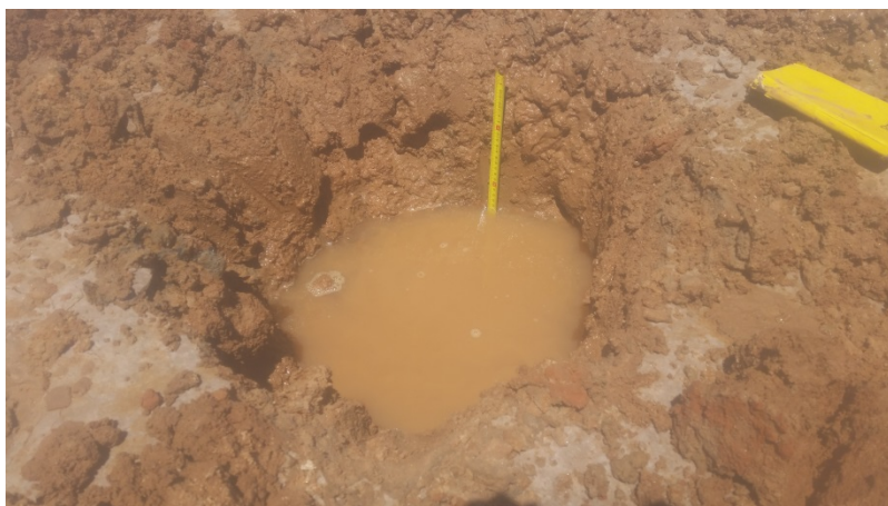
Figure 8: Brine Sampling at LIP309P1, Static water level at 0.25m
