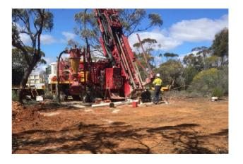
**Photograph 1.** RC drill hole PD001 is collared at the southern traverse of PEG008A
