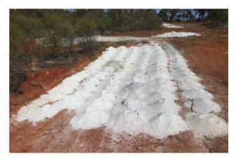
**Photograph 2.** Drill hole PD015 reached a depth of 108m, and show 103 x 1m sample piles of white pegmatite.
