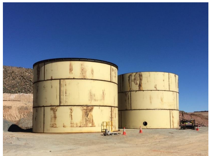
Photo 7: New leach tank to be installed after initial wet commissioning
