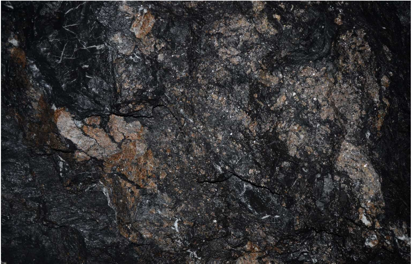
Figure 2: High-grade zinc mineralisation in cross-cut on the 940 level from where bulk samples for Metallurgical and Ore Sorting test work have been extracted
