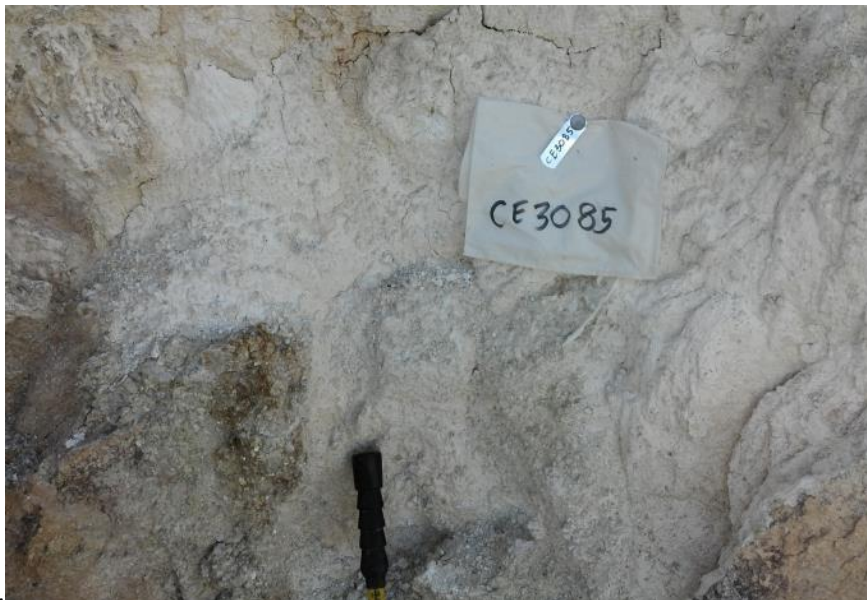
Figure 2. Pegmatite exposure in Mt Fitton Mine. Although lithium rich >1,000\text{ppm Li}_2\text{O} , much of the reactive mineralogy has been weathered to clay minerals.
