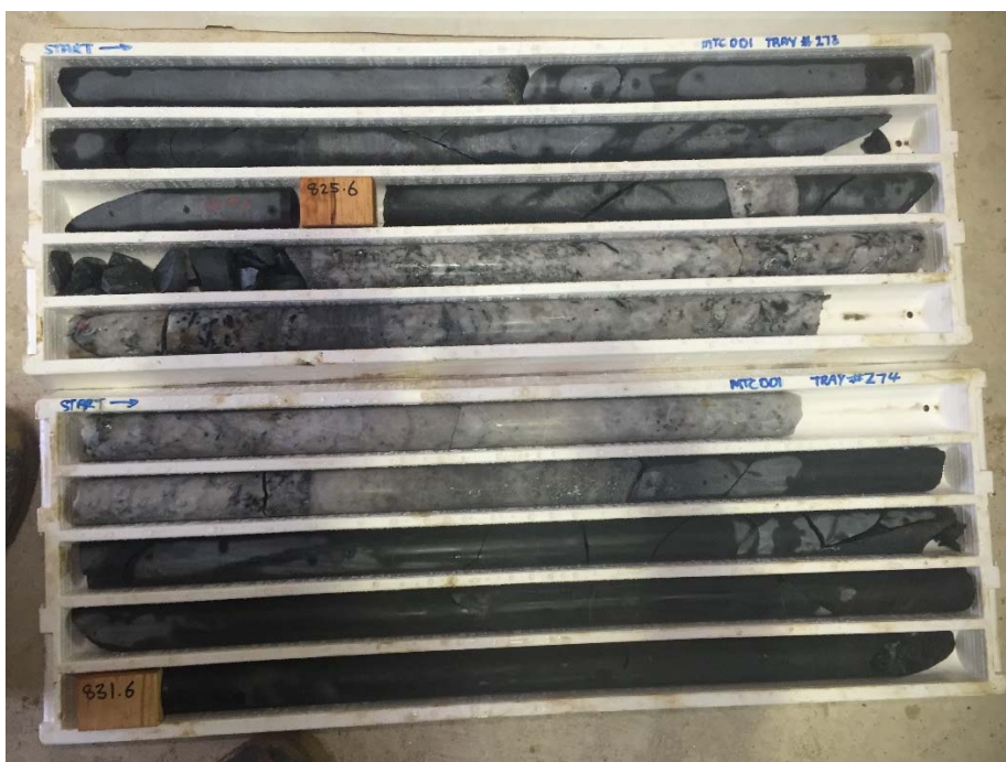
Figure 2: Fine-grained spodumene in pegmatite intersection in drill core, Hole MTCDD1W1, depth approx. 828m
