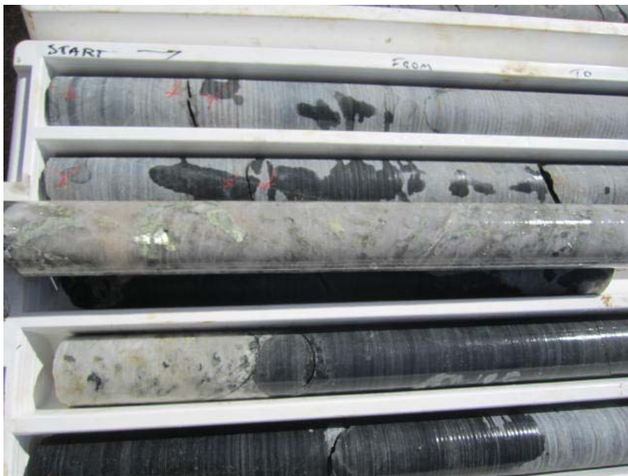
Figure 1: Pegmatite intersection in drill core, Hole MTCDD1, depth approx. 428m
