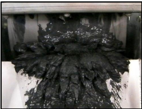
After second magnetic separation 66%Fe
