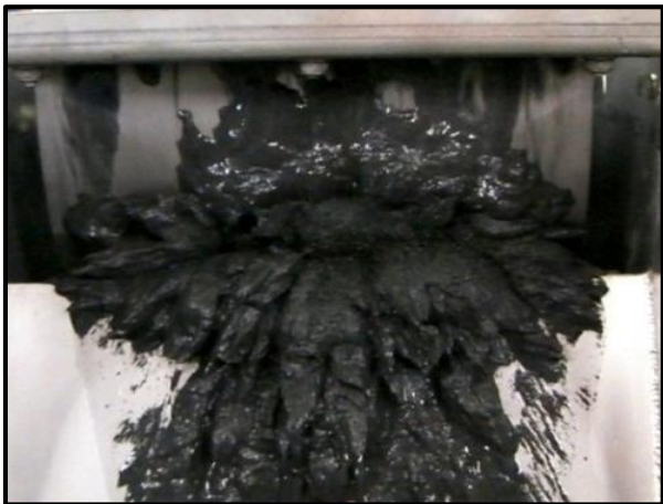
45% rejection at first magnetic separation
