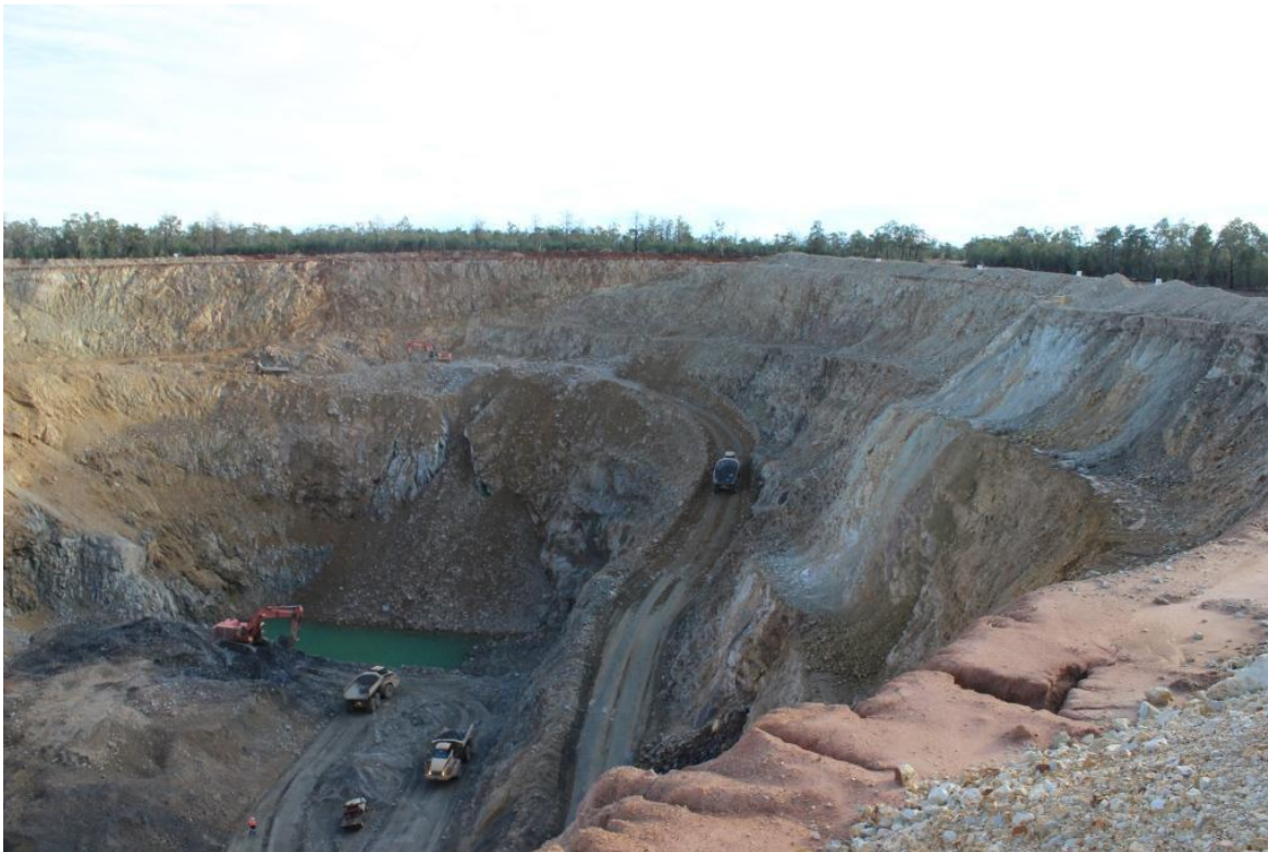
Photograph 1. Ore haulage from base of pit via re-established ramp.
