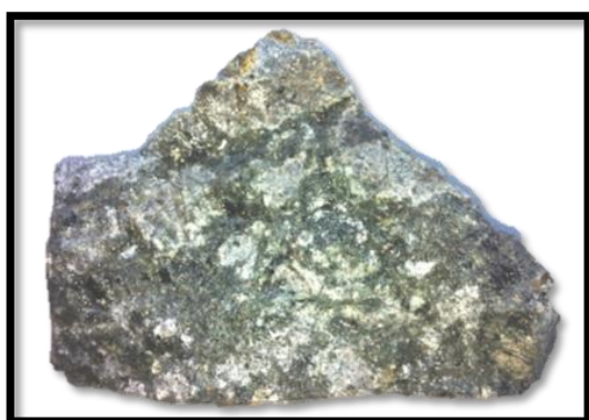
Figure 11a) Brecciated Dacitic Porphyry with disseminated chalcopryite and chalcocite from the base of the Carmelita workings (~50m below surface) on the eastern edge of Target 1. Sample assayed 3.1% Cu, 0.1g/t Au, 11g/t Ag and 200ppm Mo 1 .
