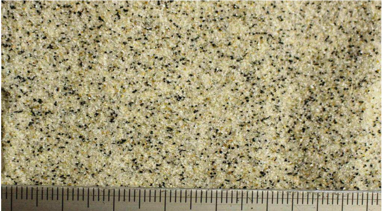
Photomicrograph of - 600 + 300 Spiral concentrate – mostly ferberite and topaz
