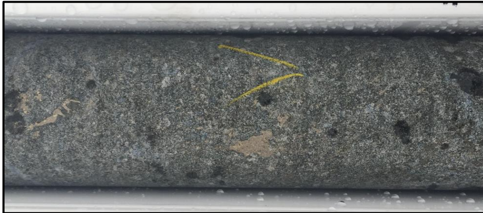
Photo 3: RKDD002-626.5m: Pyrrhotite (brown), trace pentlandite/chalcocopyrite in cumulate textured gabbro (NQ2 core)
