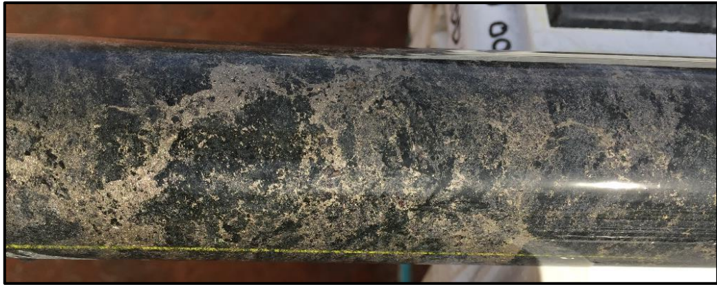
Photo 1: RKDD001-566.8m: Pyrrhotite in mafic granulite (NQ2 core)
