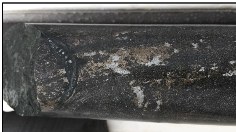
Photo 2: RKDD002-508.5m: Pentlandite (silver), pyrrhotite (brown) in mafic granulite (NQ2)
