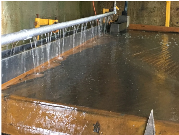
Figures 1C & 1D – Commissioning the dressing table and final 55%Sn concentrate (dried)
