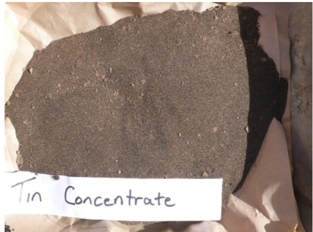
Figures 1C & 1D – Commissioning the dressing table and final 55%Sn concentrate (dried)
