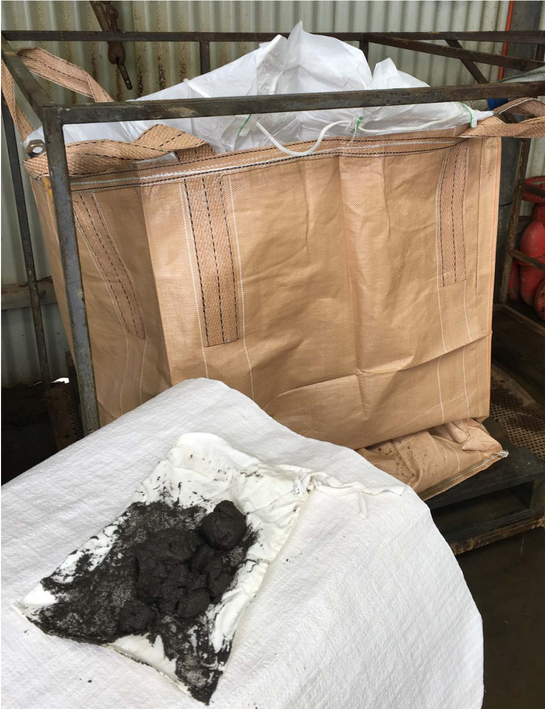
Figures 1E – Final tin concentrate and filling concentrate bag #1
