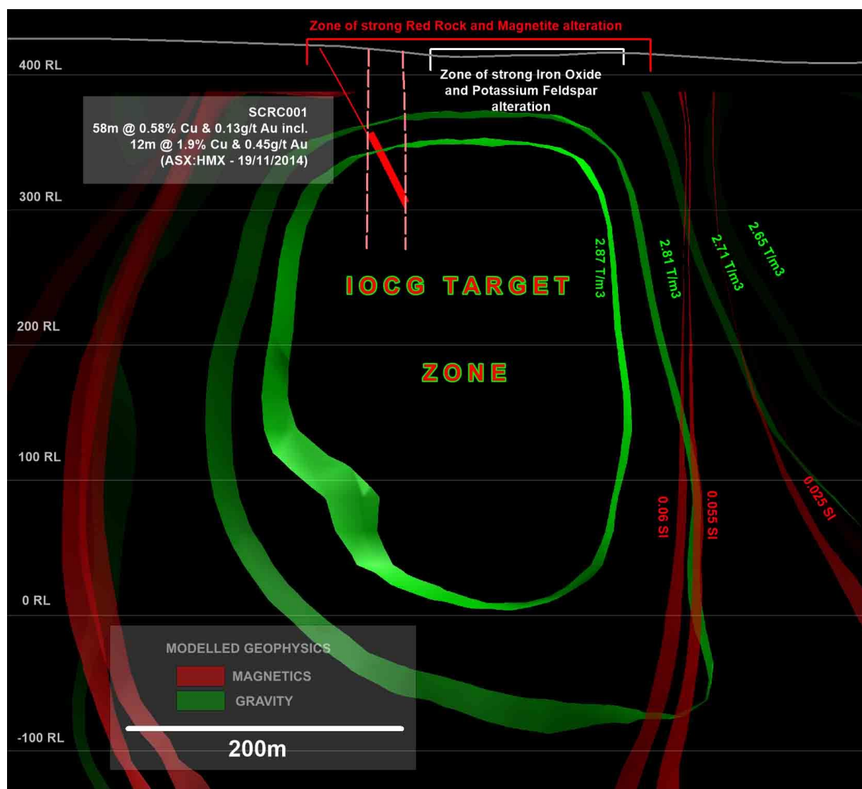
Scalper Cross Section showing magnetic and gravity modelling
