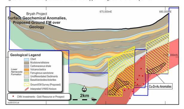
This survey is designed to locate potential Degrussa – Monty style volcanogenic massive sulphide (VMS) mineralization. It will cover a 5 km strike length of the prospective horizon with survey lines every 200 metres. About 65 line km of surveying is anticipated in the initial survey. Follow up detailed surveying will be undertaken as required.
