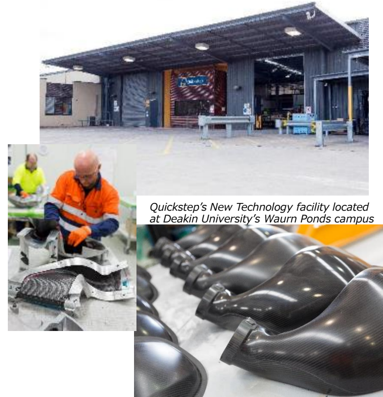
Engine compartment component developed for Ford, part weight reduced by 48%, using carbon fibre to replace thermoplastics
