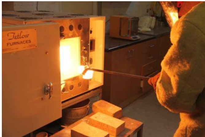
Removing deadburn magnesite from furnace
