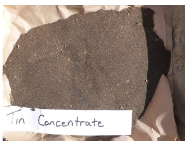
Figures 1C & 1D - Commissioning the dressing table and final 55%Sn concentrate (dried)
