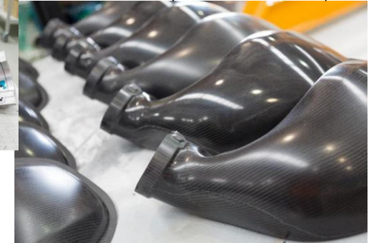
Engine compartment component developed for Ford, part weight reduced by 48%, using carbon fibre to replace thermoplastics
