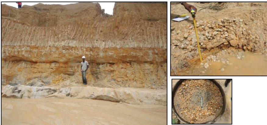
Figure 24. Bulk-sample pit MABS_023 located some 300m south of the Sumbuya Camp. Material from a well-developed basal gravel horizon (top right), with a palaeo-Sewa River stratigraphic signature (note fluvial cross-bedding), was recovered to the Sumbuya plant site for future processing. The heavy mineral assemblage is shown in the wash-sieve (bottom right).
