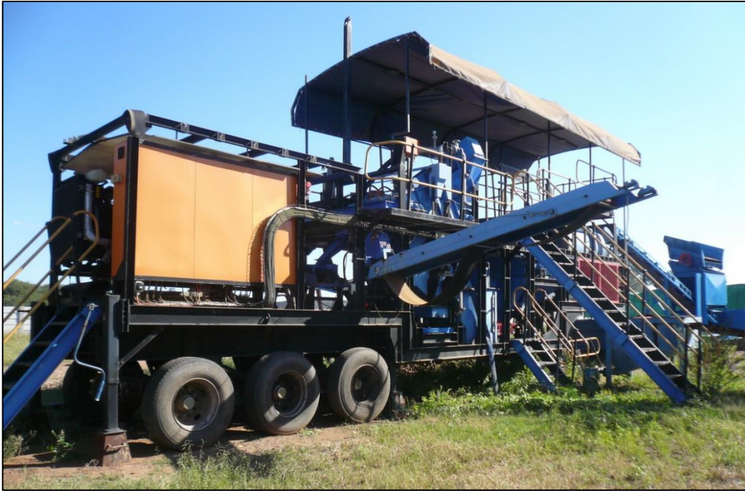
Figure 31. The new 10 tph mobile DMS plant purchased from Dynamic Machinery CC., South Africa.
