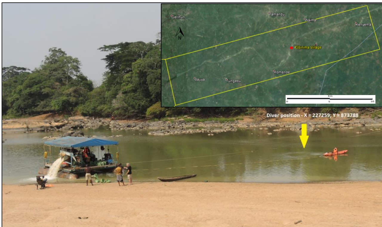
Figure 10. Photo depicting maiden dredging operations at the Sewa River Gbinima locality, EL 15/2012. Dredge position within the EL, shown inset. Of note, is the trommel debaunching sand and oversize back into the river with only the mid-sized gravel fraction being recovered for processing (refer footnote 1).
