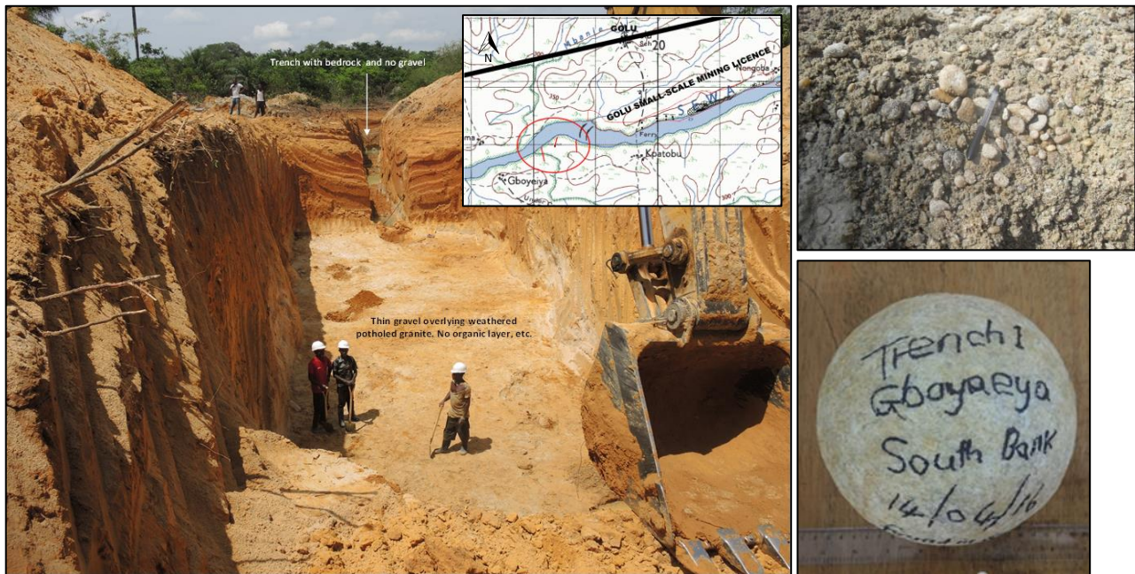
Figure 6. Gboyeyia bulk-sampling activities, Sewa River South-bank. Note rounded pebbles and boulder at right, recovered from trench 1 (main photo).
