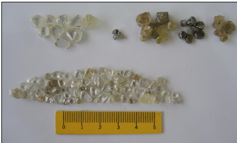
Photograph 1. Diamonds recovered from the Gbinima dredge site. The stones are of high-quality and have larger than average stone size (av. 1.2 cts/stn) when compared with the lower terrace fluvial deposits encountered at Golu (av. 0.33 cts/stn).
