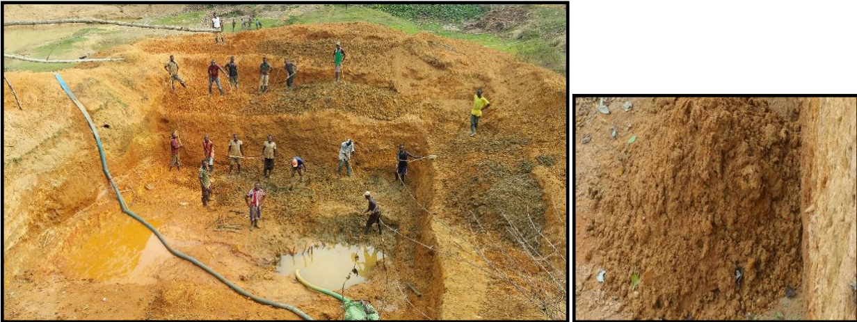
Figure 14: Exposed section in the Maina Pool bulk-sample (at left). Stockpiled gravel from the Pool (at right) was processed in the latter half of 2015.
