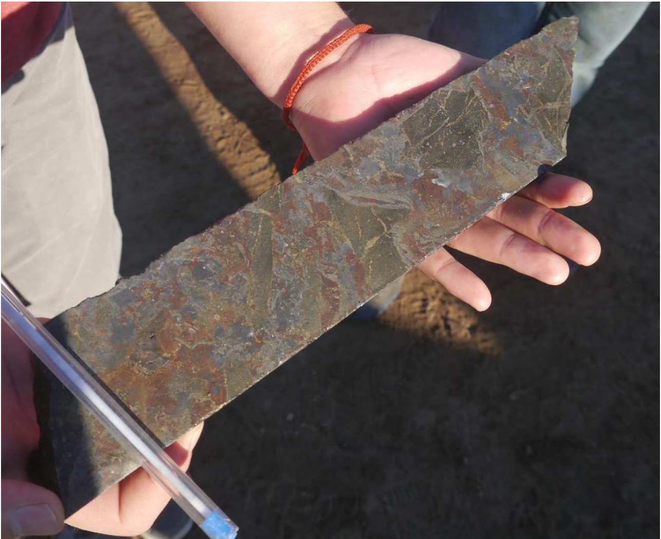
Photo 2: Drill core from Hole PTDD101 with hydrothermal breccia from the Cathedral Vein. This metre interval (119 – 120m) assayed 7.4% zinc, 14.6% lead, 631 g/t silver and 0.5 g/t gold.
