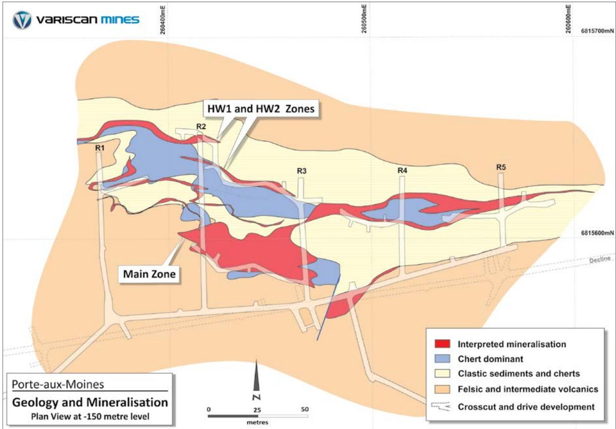
Plan view of Porte-aux-Moines deposit showing interpreted mineralised zones and underground development completed by the BRGM
