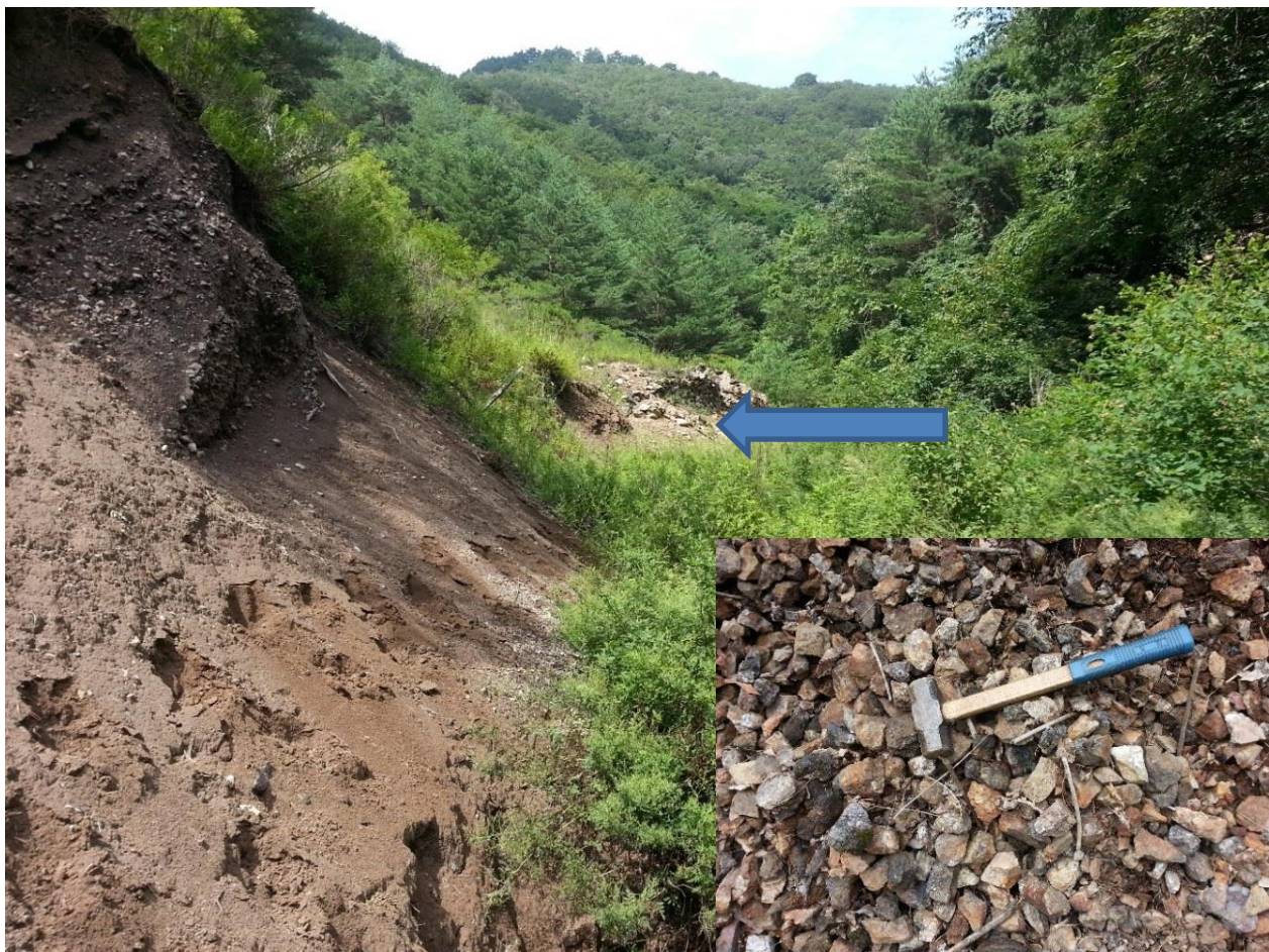
Figure 3: Slag from zinc smelting, Main Workings, Ubeong Project with close up of the slag from historic smelting site.
