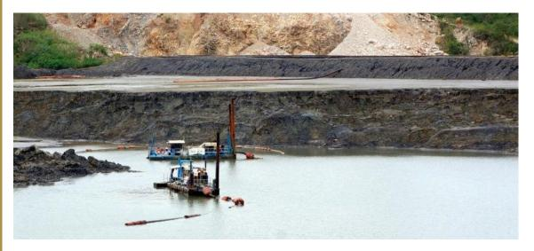
Dredging currently in coarse, higher grade material which should be typical for the balance of the resource.
