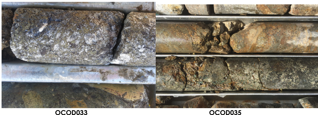
Figure 1: Massive sulphides in OCOD033 (177m down-hole, approximately 70m below surface) and OCOD035 (165m down hole, approximately 72m below surface) at the PC Project.
