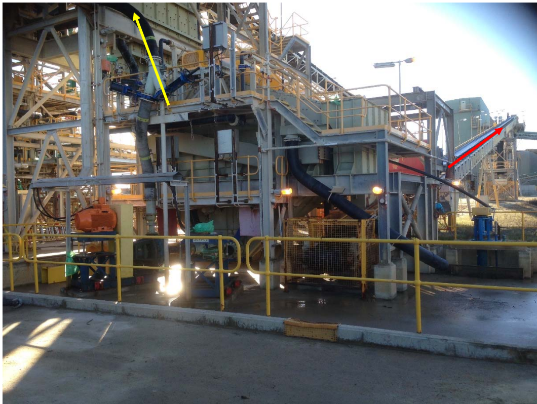
Fig 2: Discharge undersize from Feed Prep Screen transferred to the Spirals building (yellow), oversize discharged on to CV07 (red).
