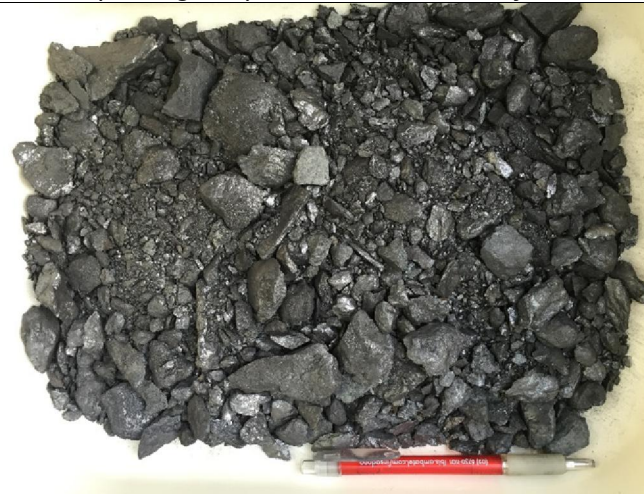
Graphite sample from underground for Met testing
