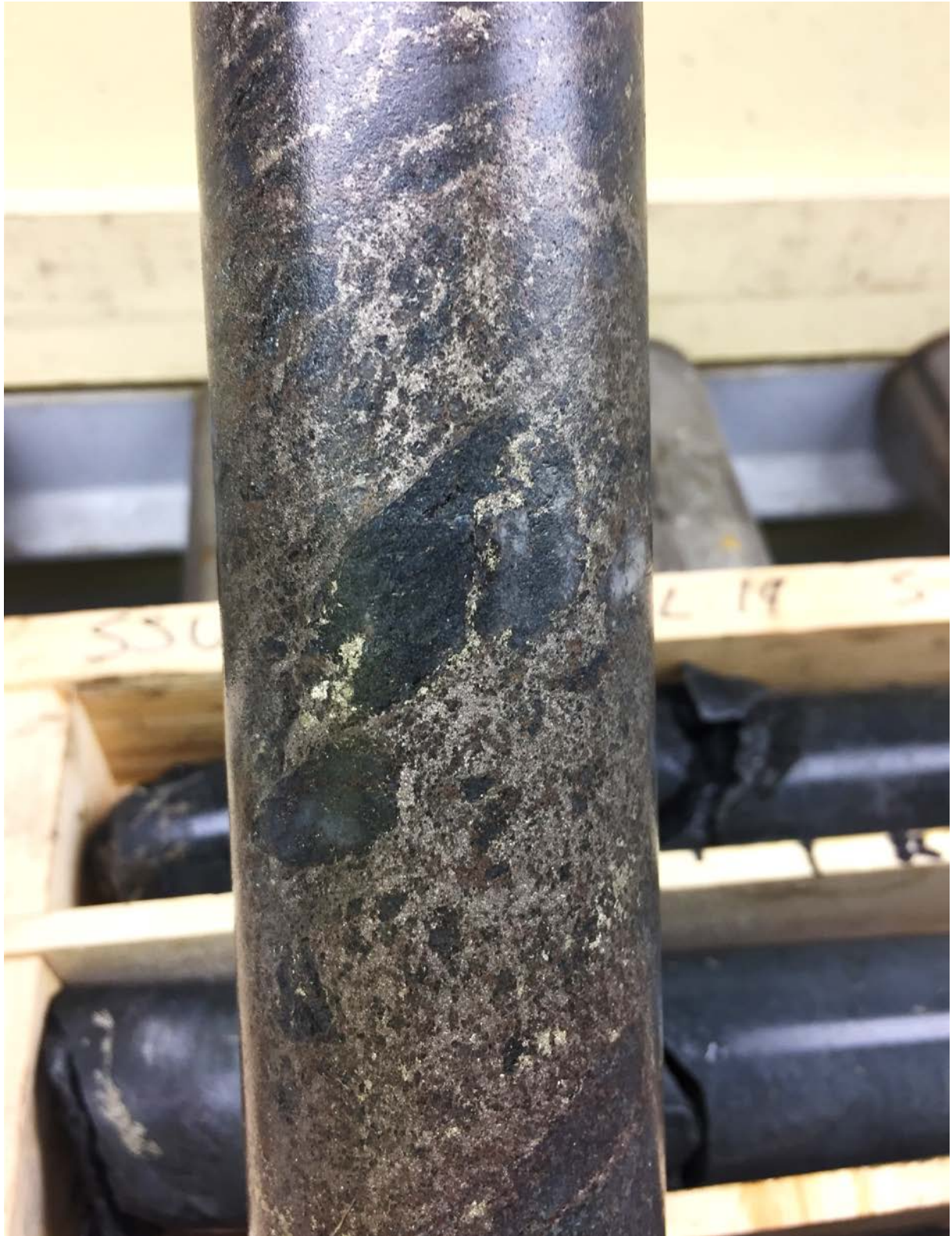
Figure 4. Photograph of massive sulphide intercept in hole SSVA160001, Svan Vit prospect, containing pyrrhotite (pale bronze brown), pyrite (brassy yellow) and sphalerite (reddish brown) with clasts of wallrock (dark grey).
