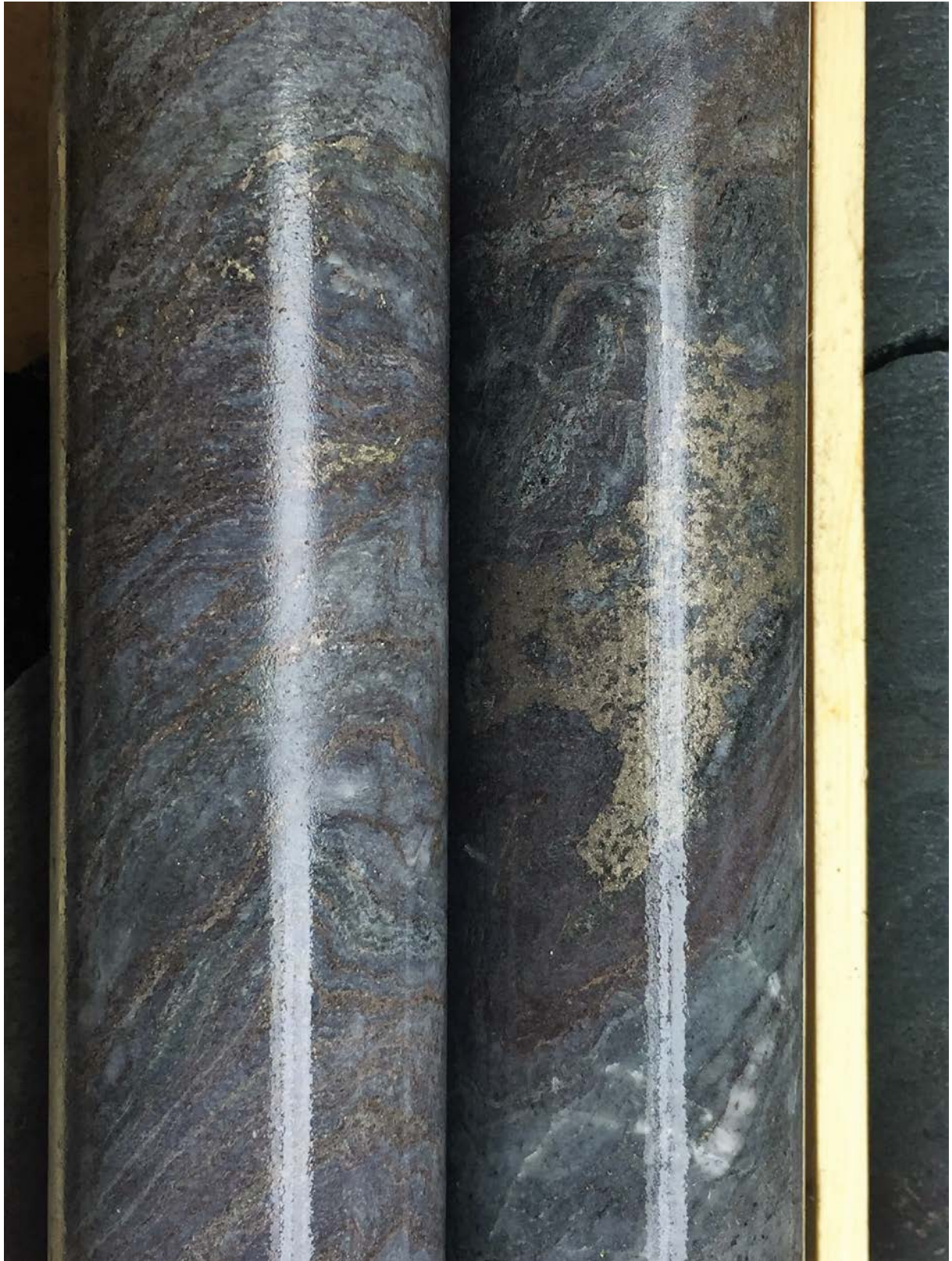
Figure 5. Photograph of core from 171 metres in hole SSVA160002, Svan Vit prospect, showing laminated sphalerite (pale pink, pale brown, reddish brown), coarse pyrrhotite (brassy yellow) and silica alteration (glassy grey to milky white).
