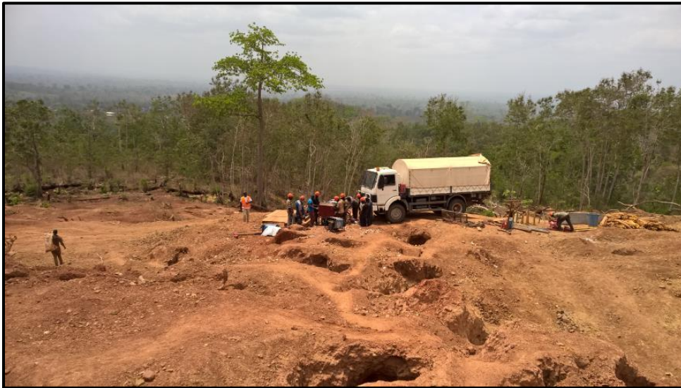
Figure 5: Photograph taken just as drill hole KOD001 was being set up. Note also the surrounding large area of recent surficial artisanal gold workings.
